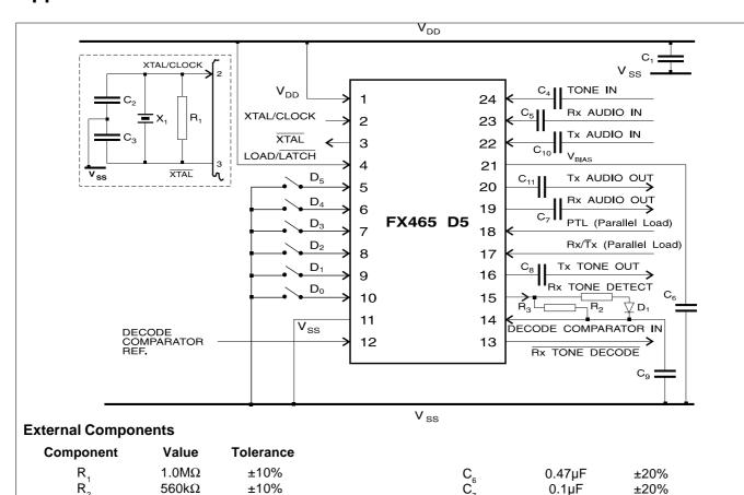
R<sub>2</sub> R<sub>3</sub> C<sub>1</sub> C<sub>2</sub> C<sub>3</sub> C<sub>4</sub> C<sub>5</sub>  $820k\Omega$ ±10%  $0.1 \mu F$ ±20% 0.1µF ±20%  $0.1 \mu F$ ±20% 18pF ±20% ±20% 0.1µF 33pF ±20% 0.1µF ±20%  $0.1 \mu F$ ±20% small signal type  $0.1 \mu F$ ±20% 4.0MHz ±0.01%
